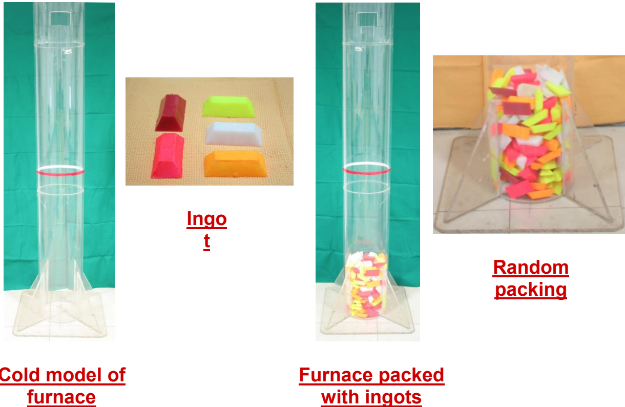
Figure 8 : Rubber Models of Cupola Furnace & Ingots used for Simulations
